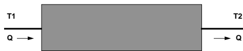
Figure 3-1. A thermal conductance with a linear relationship between heatflux, Q , and temperature difference, T1 - T2 .
